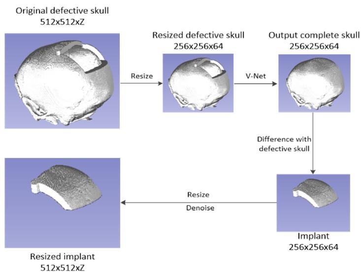
**Figure 1** – Workflow of resize method. The original defective skulls are resized to 256x256x64 and then inputted into the network. The implants are obtained via the difference of the outputted complete skulls and the inputted defective skulls. Finally the implants are resized back to the original sizes and then denoised to improve the prediction accuracy.
