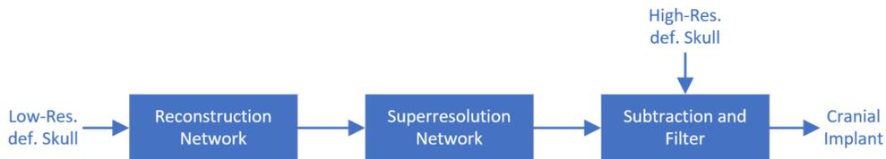
Figure 1 – Implant generation pipeline.
