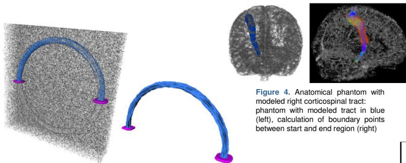
**Figure 3.** Torus-shaped software-phantom: calculation of boundary points (left), 3D object generation (right)
