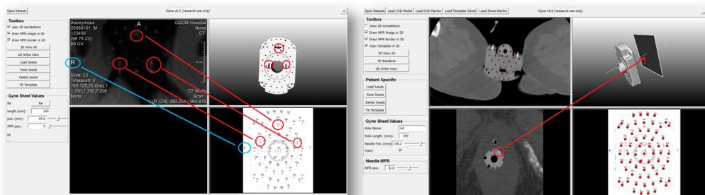
Figure 2a – Principle for fitting a gynecological template for brachytherapy with an initial CT image. The three red circles indicate corresponding needle holes in the template and the patient image. The fitting is realized via a rigid transformation between these corresponding point sets. The blue circles are used to ensure that the left and right sides of the patient and the template are matched correctly.
