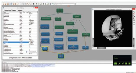
Fig. 3 The overall MeVisLab network with the *HTCVive* module and its interface, and parameters on the left side.
