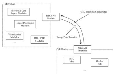
Fig. 2 High level workflow diagram showing the communication / interaction between MeVisLab and the HTC Vive via OpenVR.
