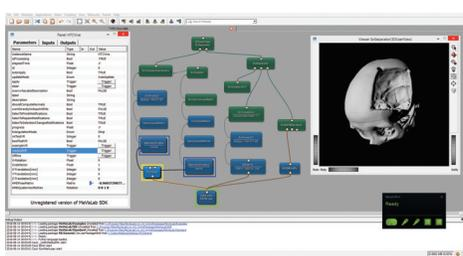
Fig. 3 The overall MeVisLab network with the *HTCVive* module and its interface, and parameters on the left side.
