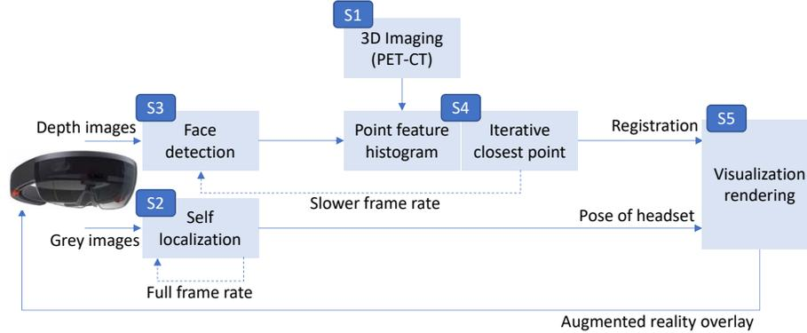
Fig. 1. Overview of the proposed five-step registration pipeline.
