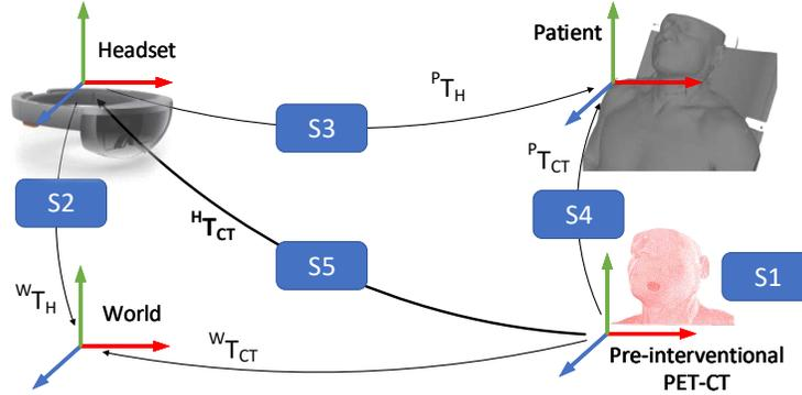
**Fig. 2.** Coordinate systems and their transformations to be computed during image-to-patient registration. The goal is to find  ${}^H T_{CT}$ , the relative pose of the PET-CT coordinate system  $CT$  with respect to the physician, denoted by  $H$ .
