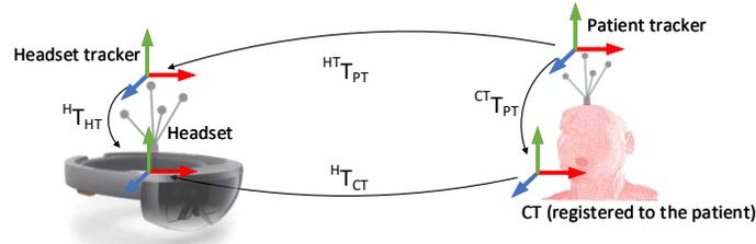
**Fig. 4.** Coordinate systems for comparing  ${}^H T_{CT}$  to  ${}^H T_{PT}$  from an external infrared tracking system.  ${}^{CT} T_{PT}$  and  ${}^H T_{HT}$  are estimated using hand-eye calibration.
