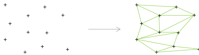
Figure 11: Triangulation process using a cloud of vertices (left) to generate a mesh consisting of triangles (right)
