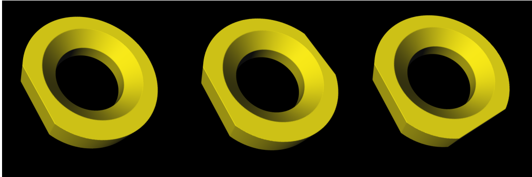
Figure 31: Shows the three ring elements of the implant provided by WEM-Load1 (left, end parts), WEMLoad2 (middle, center parts) and WEMLoad3 (right, angled part)
